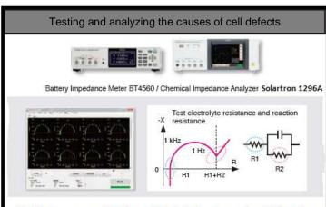
Identify the causes of battery cell defects by measuring AC impedance at multiple frequencies. For example, you can identify batteries that have issues with electrode reactions at the electrode interface by checking impedance at low frequencies. You can also extend this approach to cover multiple channels by combining the instrument with a switching system.
